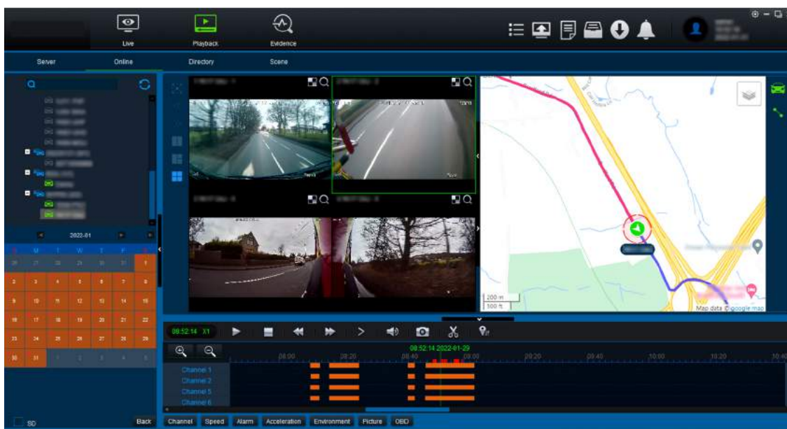
A screenshot from the web app browser interface, combining multi-channel video, mapping with routes and location, and speed & alarm events.
