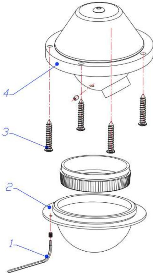
1. Use the hex key supplied (1) to loosen the hexagon socket screw (3) then unscrew the top cover (2).
