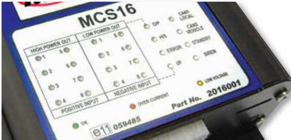
The MCS-16 has 24 diagnostic LED's on the top side of the unit, which can be used to assist the installer in finding faults, etc.
