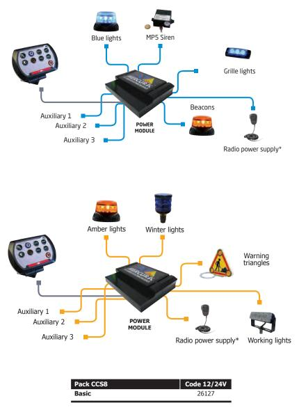
\* Permanent power supply (battery value) for radios or other power consumers.
