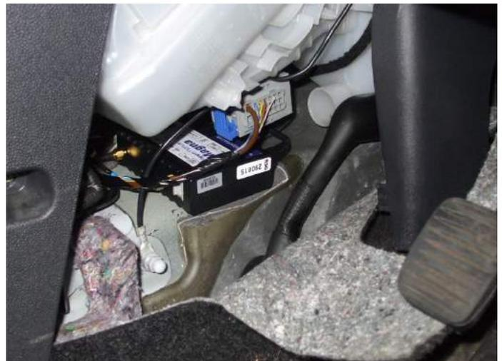
FleetMotus Magna installed into a Vauxhall Corsa
