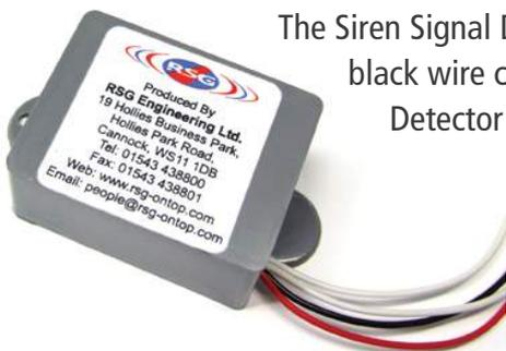
The Siren Signal Detector is connected via the two whites onto the Siren Speaker Wires the black wire connects to ground and the red wire connects to the IDR. The Siren Signal Detector fits on to the vehicle backboard.
