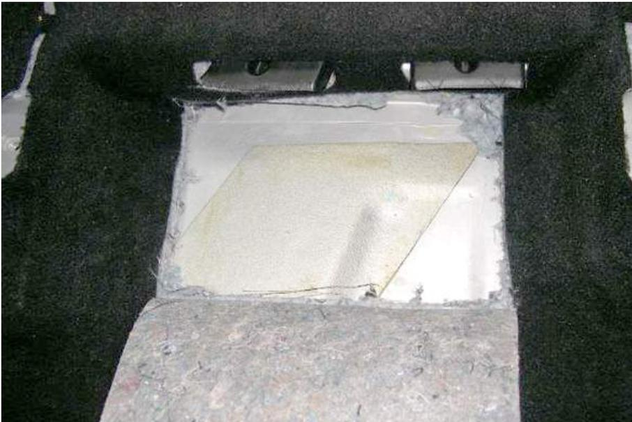
When you are ready to install the unit please use a suitable method of fixing to the floor pan of the vehicle. Methods to consider are: double sided sticky foam, hook and loop or any other suitable solution. Be aware that the FleetMotus device may be removed and refurbished so the fixing method must not damage the device.
