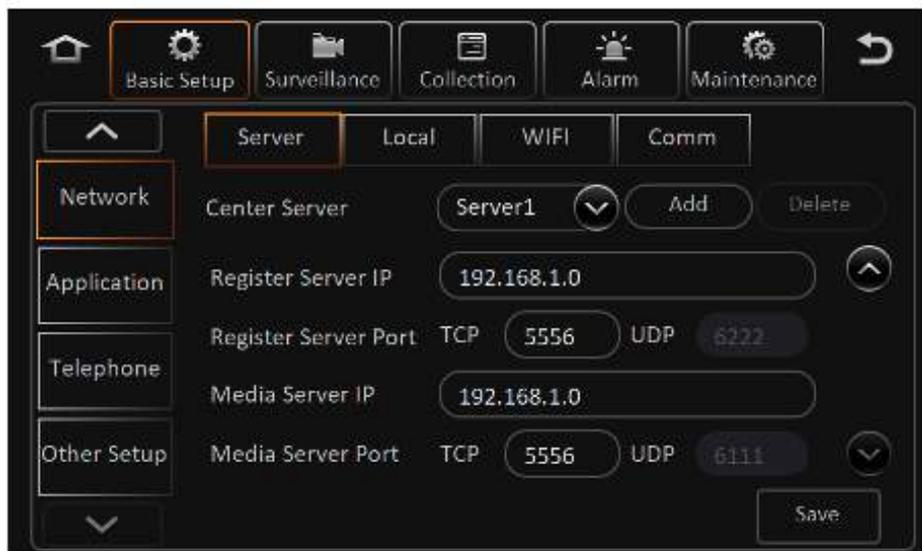
The device can connect to multiple servers at the same time according to the configuration. By default, one server is connected. It supports adding or deleting servers manually. Servers whose information can be reported include the CEIBA2 server, maintenance server, FT platform, and customer platform.
