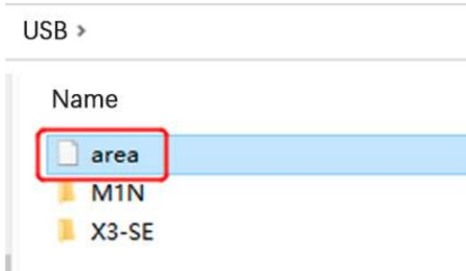
Import: Place the Geo-fence file in the root directory of a USB flash drive and tap Import to import the file. (It can also be issued remotely via the CEIBA platform.) Note: The Geo-fence is applicable to all models.
