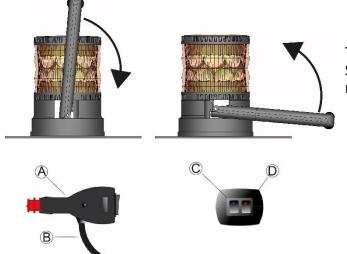
The surface of the pavilion on which the GYROLED® STICK is to be installed must be flat and clean so as not to affect the adhesion of the assembly.
