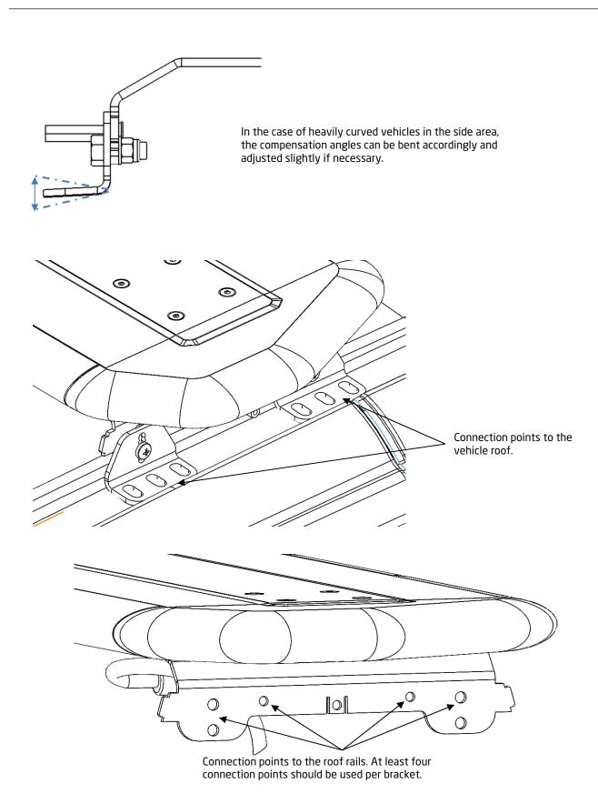
Liquid screw locking must be used for all screw connections where no nut with a clamping part is used.
