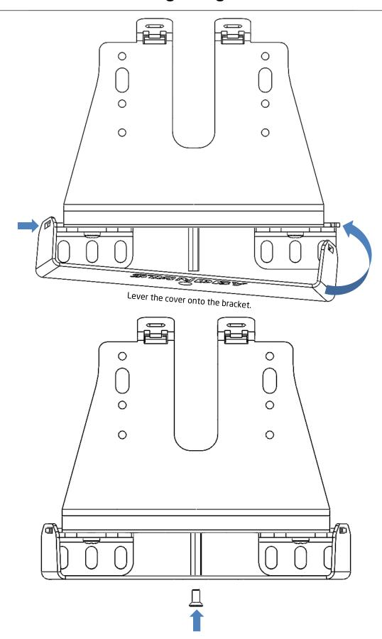
Tighten the screw (torque 2-3Nm, use liquid screw locking agent).
