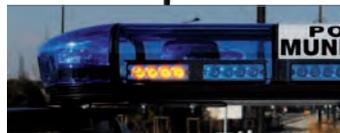
**Warning :** Warning mode, the complete amber beacon light unit flashes at the same time (Available on lightbars with amber beacon lights)
