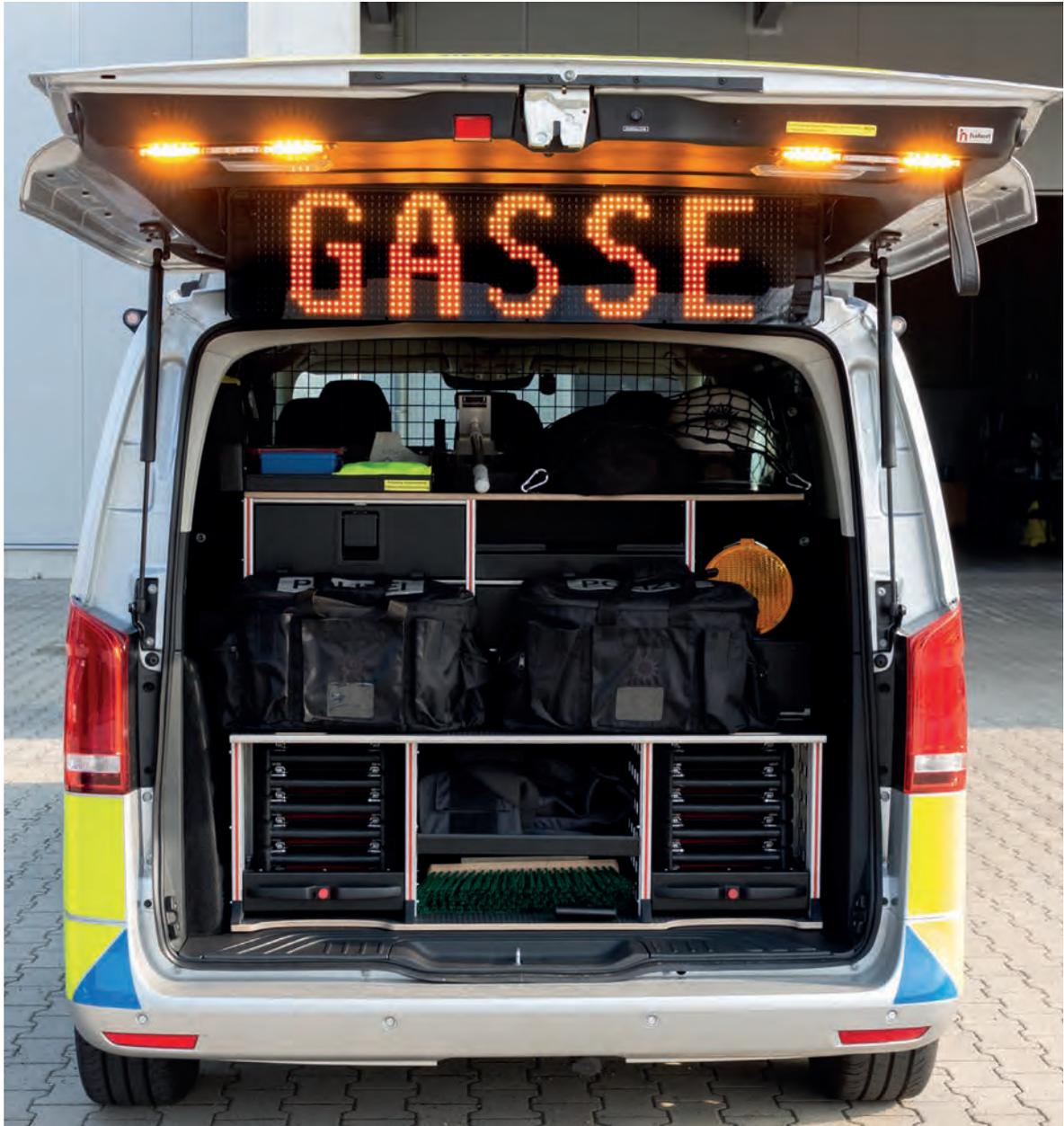
The first full matrix display that complies 100% with the police car guideline. Stop signaling texts (*ASG*) are shown in red font, information signaling texts (*ISG*) are shown in yellow font without limits on the sides.
