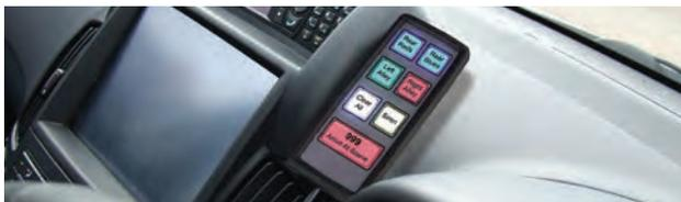
**MCS Control Units are user programmable devices for managing hazard warning lights and power related functions on Emergency Services vehicles. Standard units incorporate a 100 Watt siren with both UK and European tones. These devices incorporate a host of discrete on/off and various data protocol inputs and outputs to control a wide variety of applications.**
