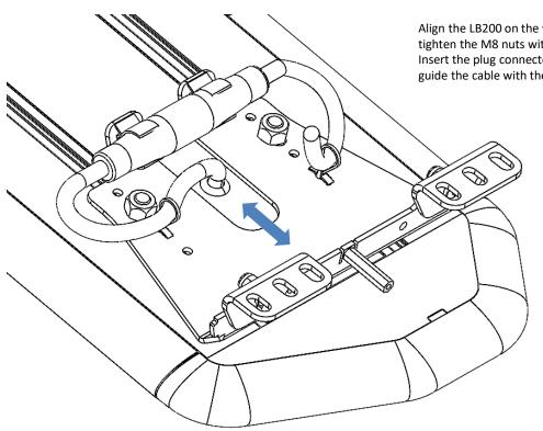
Align the LB200 on the vehicle roof by moving the brackets and tighten the M8 nuts with 6 Nm. Insert the plug connector into the retaining clips provided and
