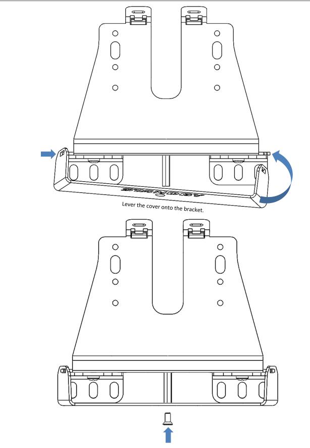
Tighten the screw (torque 2-3Nm, use liquid screw locking agent).
