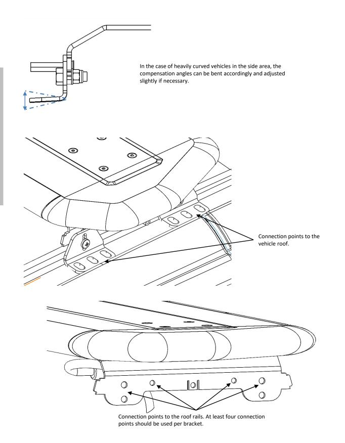
Liquid screw locking must be used for all screw connections where no nut with a clamping part is used.
