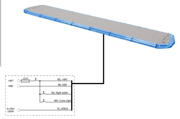
vehicle side; cables that are not required NOT shown!
