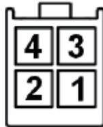
Pin 1: Logic input 2 is an input to the "-BATTERY" which does not wake up the system. A handbrake information can be connected to it.
