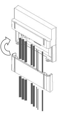
• Place the module and press firmly to connect the fastening strips.
