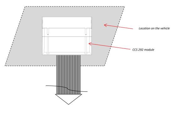
Harnesses to equipment, power supply and control box.
