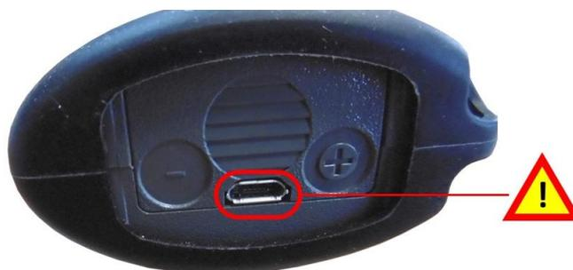
**LE PORT USB SITUE SOUS LA POIGNEE N'EST PAS UTILISE ET NE DOIT ABSOLUMENT PAS ETRE CONNECTE POUR RECHARGER L'APPAREIL.**
