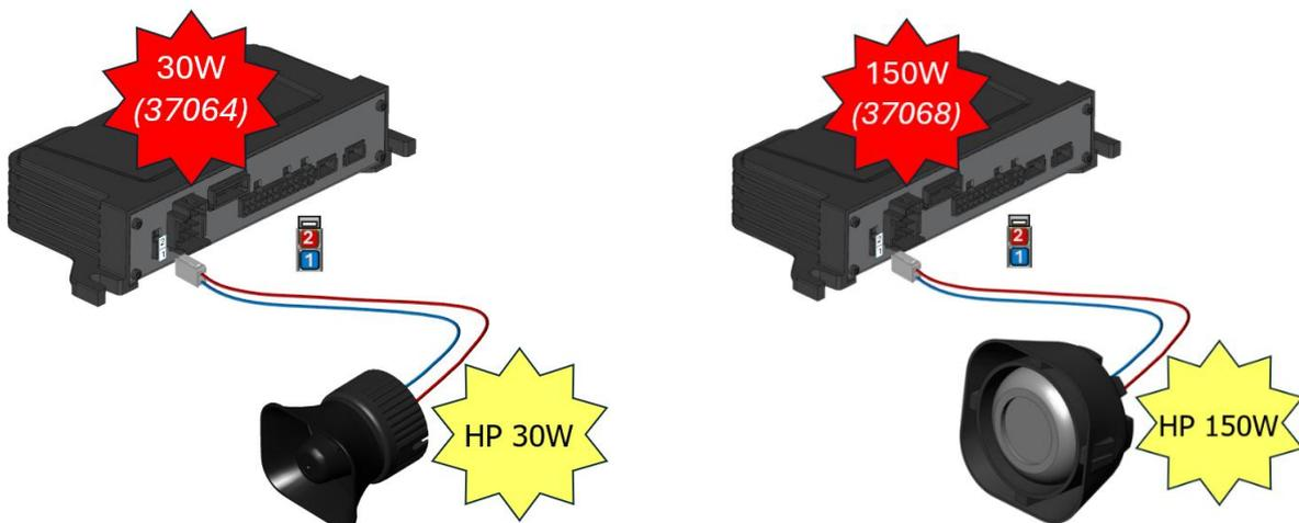
\*LE SIGNAL SONORE ETANT UN SIGNAL ALTERNATIF, LA POLARITE DU BRANCHEMENT IMPORTE PEU.
