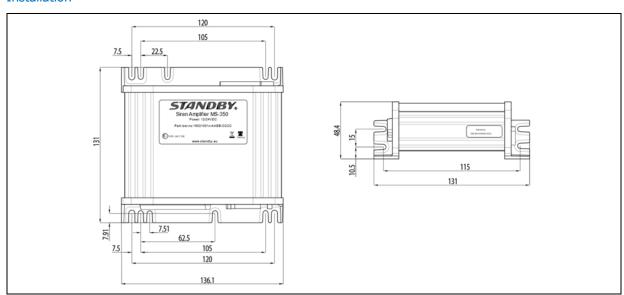
The Control-Unit can be installed as desired in the vehicle interior. Due to the housing design, the Control-Unit can be variably attached and connected to the vehicle with four screws. Care must be taken to ensure good accessibility of the connectors.
