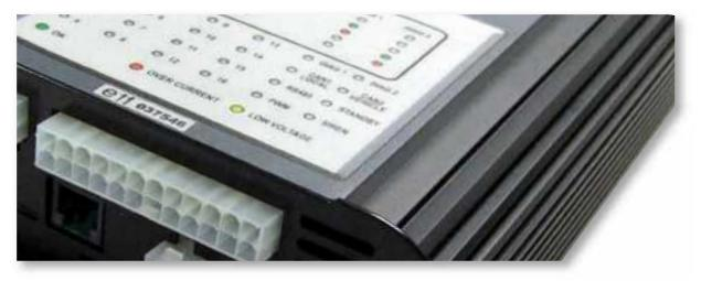
The MCS-32 has 24 diagnostic LED's on the top side of the unit, which can be used to assist the installer in finding faults, etc.
