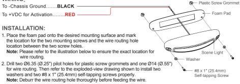
3. Feed the wires through the foam pad and wire routing hole and mount the scene light with the supplied self-tapping screws.
