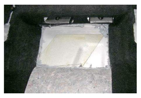
When you are ready to install the unit please use a suitable method of fixing to the floor pan of the vehicle. Methods to consider are: double sided sticky foam, hook and loop or any other suitable solution. Be aware that te FleetMotus device may be removed and refurbished so the fixing method must not damage the device.
