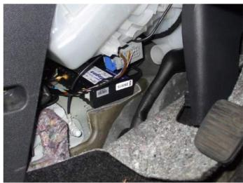
FleetMotus Magna installed into a Vauxhall Corsa
