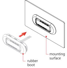
**WARNING:** When inserting into mounting hole, exert force only on the rubber boot.
