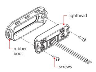
**NOTE**: Do not over-tighten the screws.
