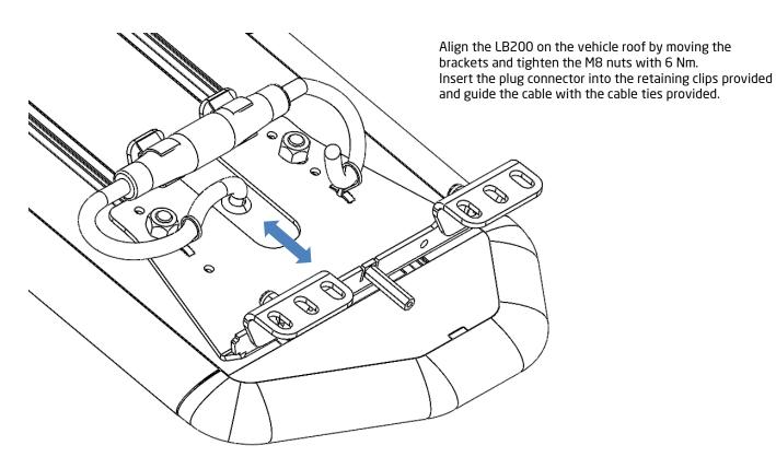
Adjusting the height and aligning the brackets using the compensation angles. The support surface of the bracket must be parallel to the road surface.
