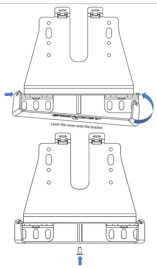
Tighten the screw (torque 2-3Nm, use liquid screw locking agent).
