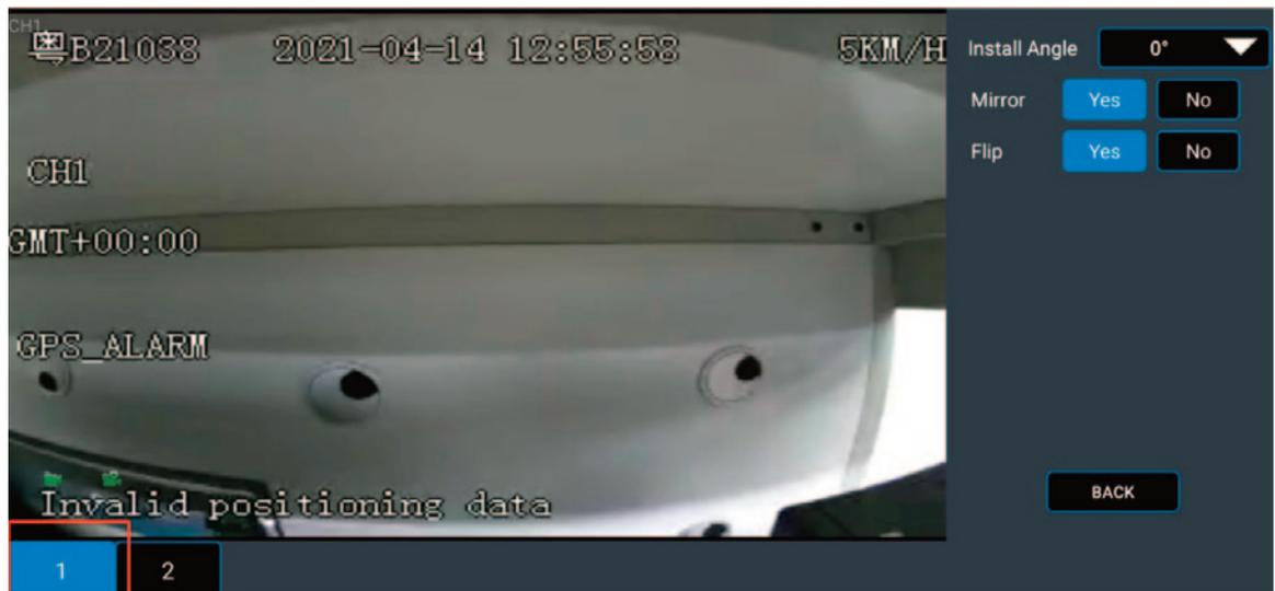
In the lower left corner of the screen, select the target channel to set the rotating angle of the camera in this channel, and enable or disable mirroring and flipping for the camera.
