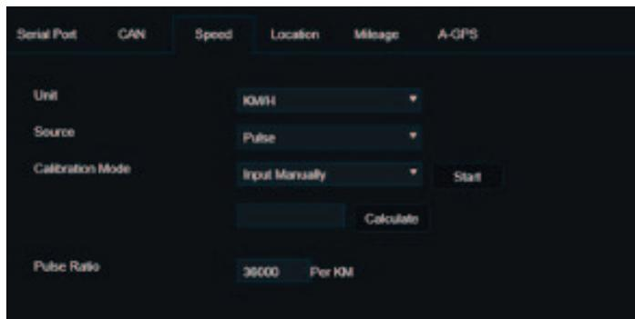
Calibration Mode: can be set to Input Manually or Automatic Correct.
